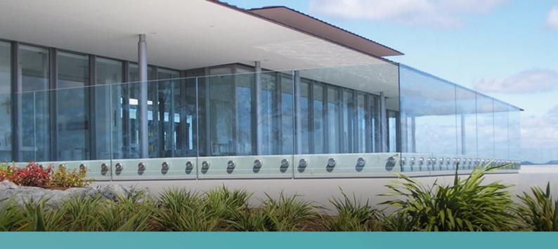
Mono is a strong and durable point-fixed frameless glass balustrade system. It features anchors that are securely bolted through the glass panels. This provides extra support and rigidity. The compactness of the bolts and their covers reduces the visible hardware, ensuring a modern style without compromising the security and reliability of your balustrades.
